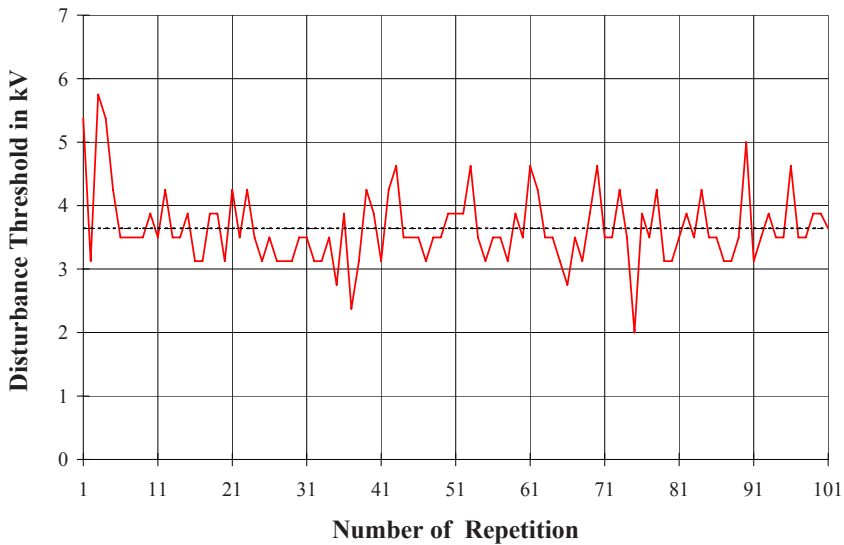
Fig. 11.2 Variation of the assessed disturbance threshold of a PLC against ESD during repetitive testing
